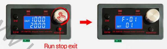
In the running interface, the rotary encoder adjusts the speed, CW button-forward rotation, CCW button-reverse rotation, RUN/STOP button-operation stops and exits. Long press the encoder to enter the menu settings.
